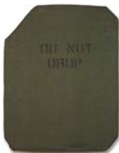
Old style aluminum oxide ceramic plate
