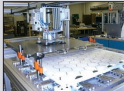
Semi-automated Armor Ceramic Assembly
