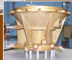
Tailrotor Gearbox After Repair
